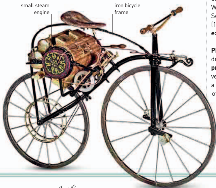
Early motorcycle Dating from between 1867 and 1871, Pierre Michaux's bicycle was powered by a small steam engine. It is thought to be the world's first motorcycle.
