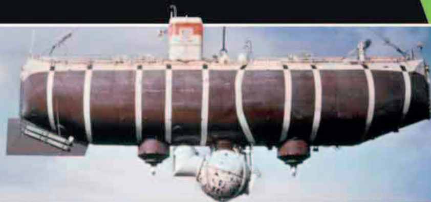
The submersible Trieste was designed to withstand the immense pressures of the deepest part of the Marianas Trench. Until 2012, it was the only manned vessel to get there.
