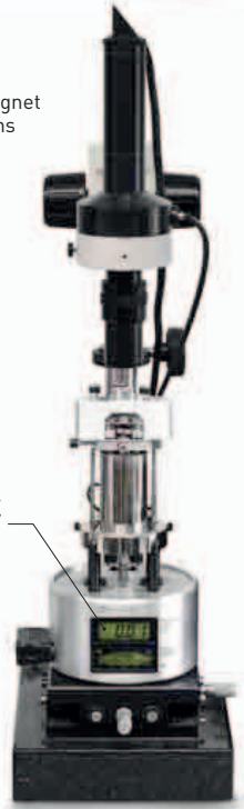
Atomic force microscope c.2000 Developed from the scanning tunneling microscope in 1986, this scans objects with an atom-sized probe and is one of the most powerful microscopes available today.
