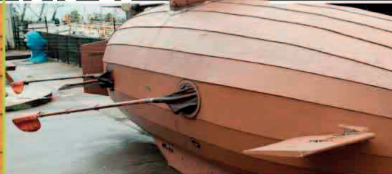
This reconstruction of Drebbel's submarine, the first navigable underwater craft, is complete with fins, a rudder, and watertight portholes for oars.
