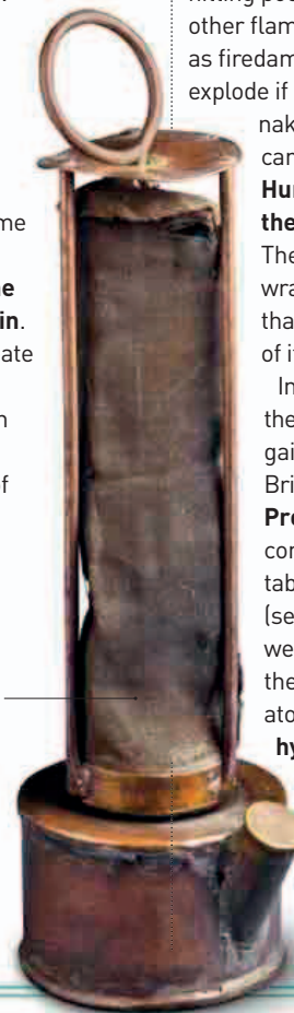
wire mesh prevents flame from igniting mine gasses
