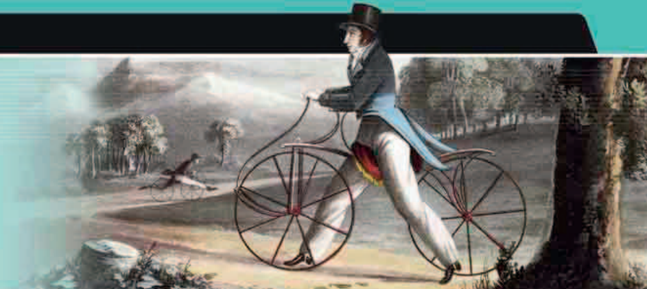
Karl von Drais's Laufmaschine (running machine) was a forerunner of the bicycle and the first two-wheeled form of personal transportation.
