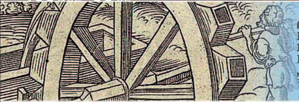
A medieval depiction of a Vitruvian undershot waterwheel. Operated with a hand lever, the buckets fill with water as the wheel rotates and the buckets dip into a water source. The water is deposited at the top.
