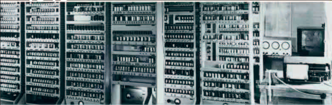
EDSAC was one of the first recognizably modern computers in terms of design, but it nearly filled a room and needed 60 in- (152 cm-) long tubes of mercury to help with memory storage.
