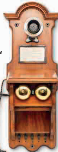
Early payphone 1905 By the 20th century, "payphones" were installed in public places. Several phones would be connected, with calls being directed by operators at a single exchange.
