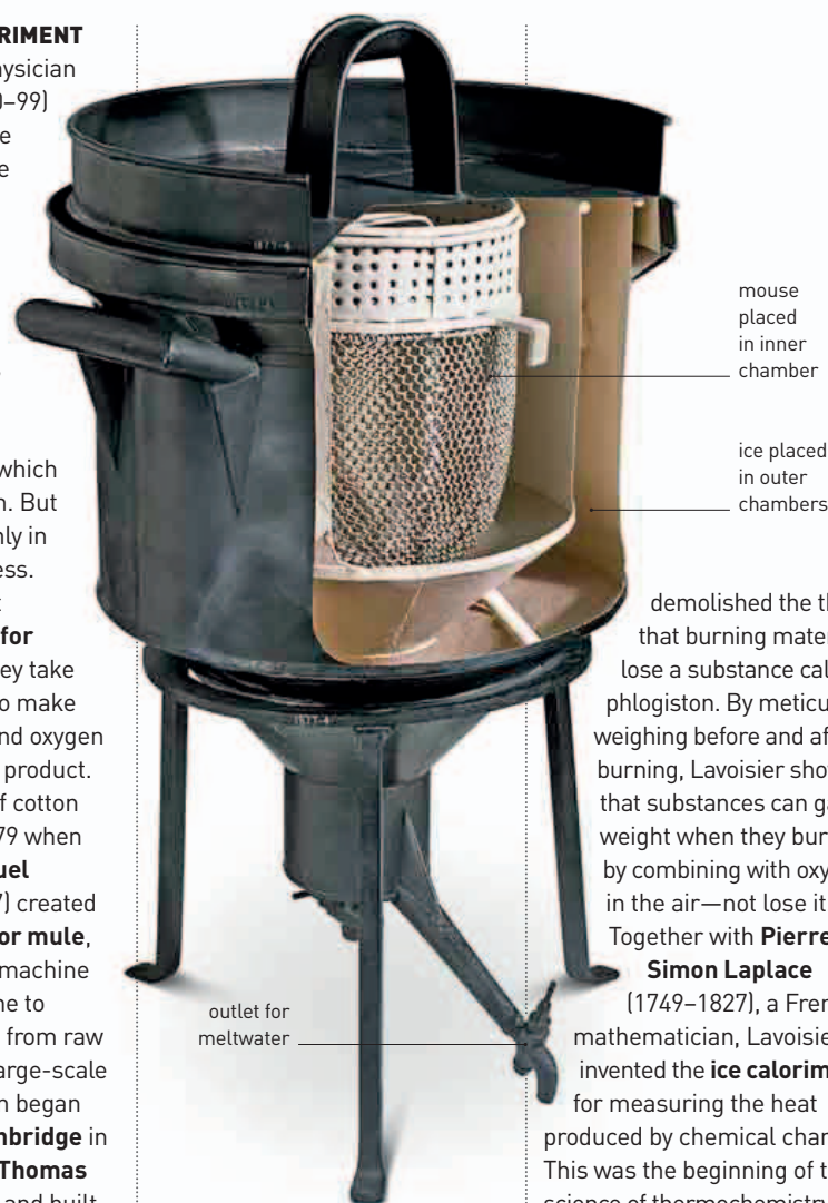
Lavoisier-Laplace calorimeter Heat produced by a mouse placed in the inner chamber was measured by the volume of water produced by melted ice in the outer chambers.
