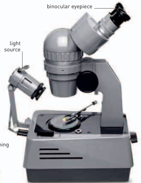
Polarizing light microscope c.1980 Polarizing filters—which line up light vibrations in one direction—are used in microscopes to study the optical properties of crystal.
