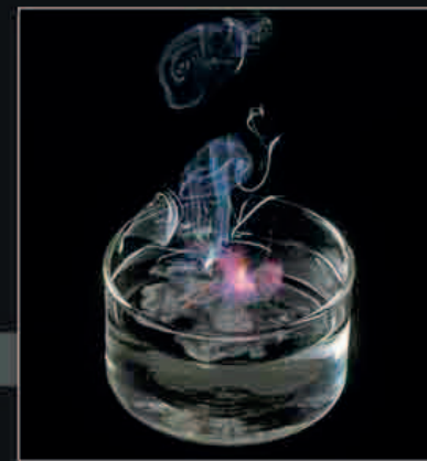
POTASSIUM IN WATER When potassium reacts with water, hydrogen gas is released. The reaction also produces heat, which ignites the hydrogen.
