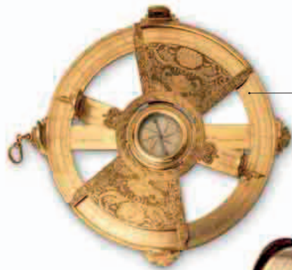
Circumferentor 1676 Used by surveyors before the invention of the theodolite, the circumferentor measured angles and could be used horizontally and vertically to calculate distances.
