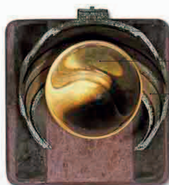
Parheliometer 1881 Hours of sunshine can be recorded on a parheliometer, in which a glass ball focuses the Sun's rays onto card so that the Sun's passage leaves a scorch trace.
