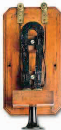
Bell's electric telephone 1876 Alexander Graham Bell's telephone transmitted sound using electrical signals. As the signal reached the receiver, a metallic disk would vibrate, producing soundwaves.
