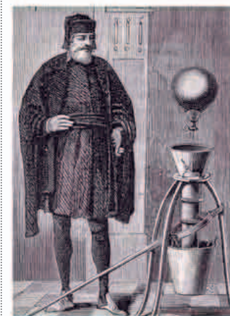
Piston-operated vacuum pump Using an elaborate piston system, Otto von Guericke created a vacuum inside two joined hemispheres, called the hemispheres of Magdeburg, after his hometown in Germany.
