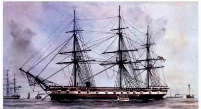
HMS Challenger Launched on February 13, 1858, HMS Challenger was primarily a sailing ship, but was also fitted with an auxiliary steam engine.
