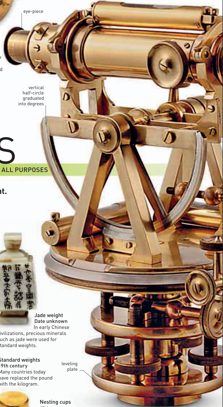
Brass half-circle theodolite 19th century A theodolite measures horizontal and vertical angles and is an important tool in surveying. The instrument's telescope is focused on a distant object, the position of which is determined with respect to horizontal and vertical scales.
