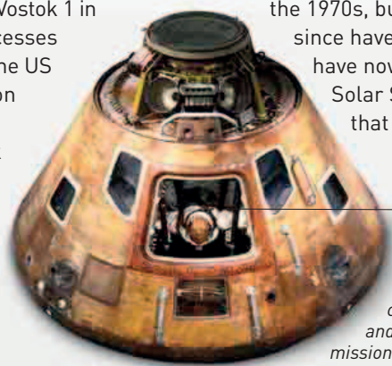
hatch through which astronauts entered and exited module
