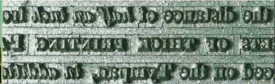
William Ged's stereotype printing process involved making a copy of the typeset page from a mold, so the copy could be used again and again for reprints.
