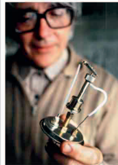
James Lovelock holds ECD The electron capture detector (ECD) picked up the tiniest amounts of electron-binding chemicals in the atmosphere, such as the chlorine in pesticides and other compounds.
