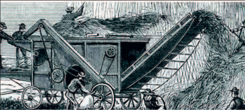
Andrew Meikle's threshing machine brought to an end the age-old practice of separating grain from stalks and husks with a hand flail.
