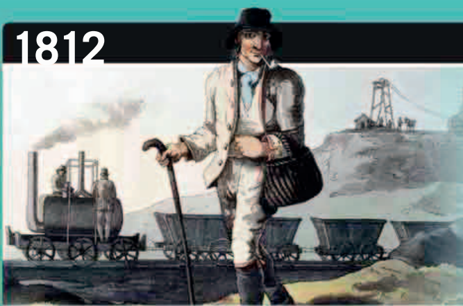
A coal train is hauled by steam locomotive Salamanca at the Middleton Colliery Railway, UK, in 1814.
