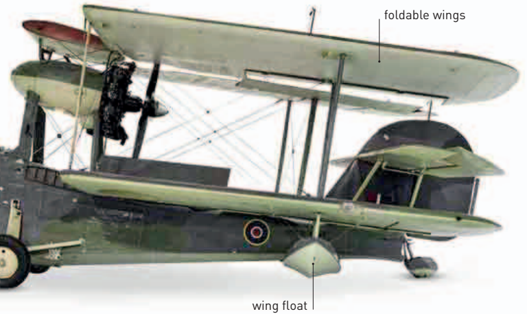
Supermarine Walrus 1935 Used for survey missions during World War II, the Walrus could be catapulted into the air from the deck of a ship. It could also land on water and be lifted back aboard.
