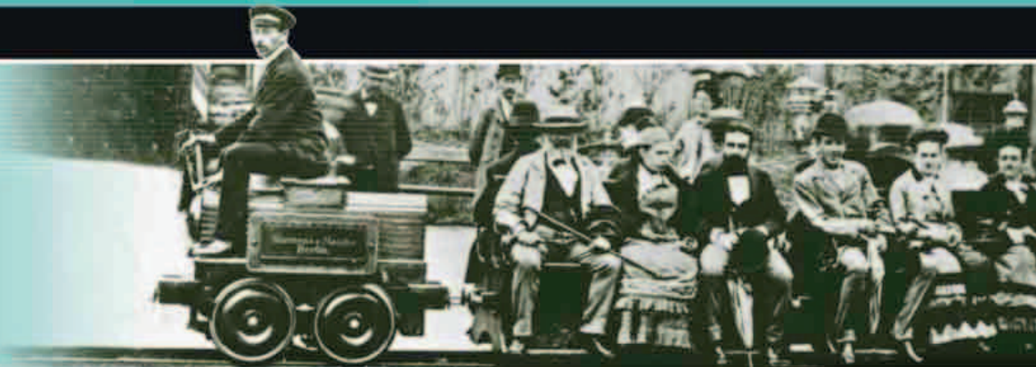
This photograph shows people traveling on carriages pulled by the Werner-Siemens locomotive, which was demonstrated at the Berlin Trade Fair in 1879. This locomotive was the first to be powered by electricity.
