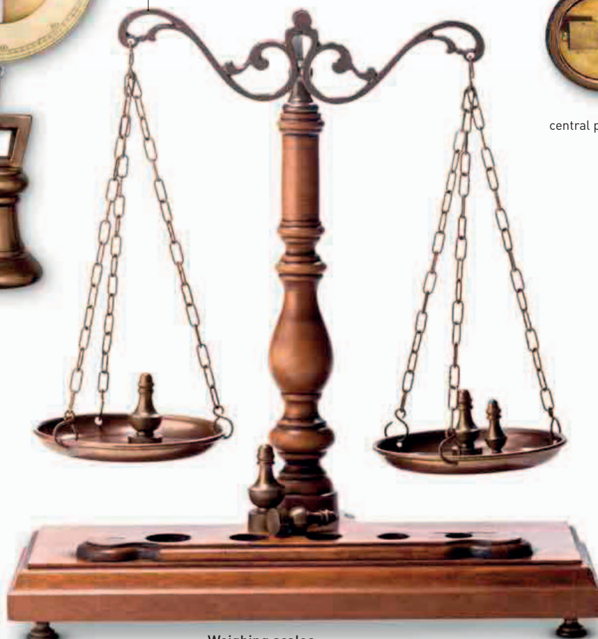
Weighing scales 18th century Scales determine an unknown weight by counterbalancing it with known weights until equilibrium is achieved.
